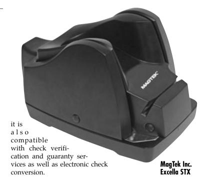
After the check is fed into the device, the front is scanned; the MICR (magnetic ink character recognition) line is processed; the back is endorsed, the front is franked, or voided; and then the back of the check is scanned.
