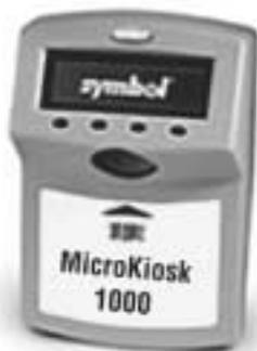
The MicroKiosk features the latest rotating omni-directional laser bar code scanning technology, 32-bit Motorola microprocessor, international language support and choice of host connectivity options, including Spectrum24 11 Mbps wireless LAN and hard-wired Ethernet support.
